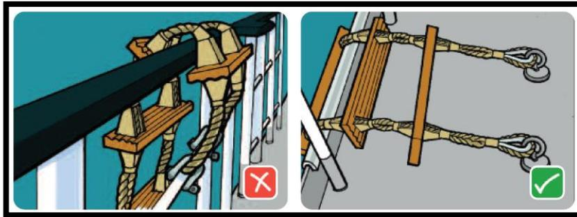
Securing pilot ladder with shackles properly on eye plates. The purpose is that the load is taken by the ropes.
